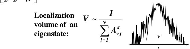
Average spacing of squared eigenfrequencies of NMs within the range of a localization volume:  $d_K \approx \frac{\Delta_K}{V}$
